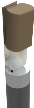
Figure 5.3: A rendering of the float sensor configuration with one side panel cut away to show the switch embedded in the body.
