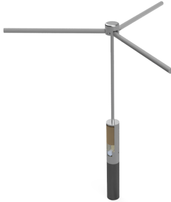
Figure 5.4: A rendering of the extended arms to brace against the walls of the cylinder.
