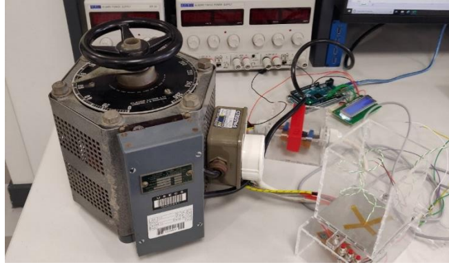
Fig. 12. A Variac autotransformer set to output 60V AC.
